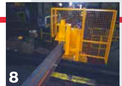
5-8 Elektromotorische Trägerwendevorrichtung für Walzprofile. Electromotive beam turning equipment for rolled steel sections.
