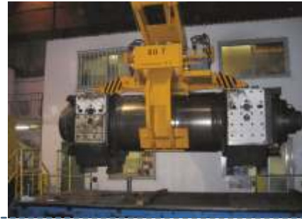
Image shows a lifter with hydraulically operated stabilizers for the chocks, SWL 60 tons
