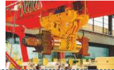
Image shows an electro-hydraulic operated WR lifter with chock stabilizers, SWL 25 tons
