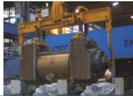
Image shows a lifting beam with J-hooks and electromotive chock stabilizers, SWL 60 tons
