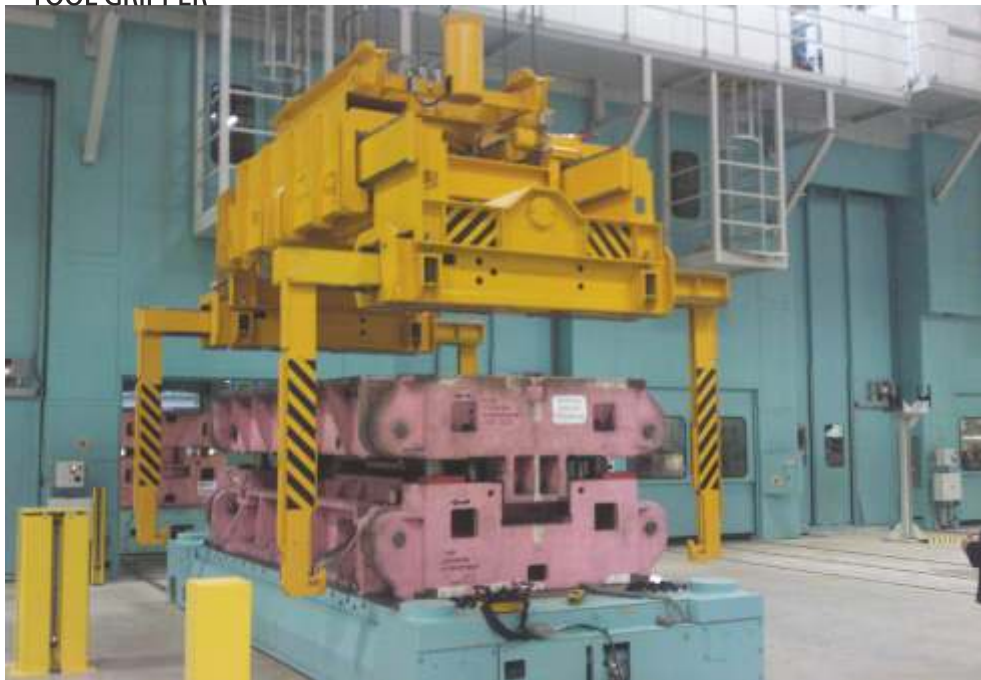
Electromotive tool gripper with spindle drive and slewing gear to handle
